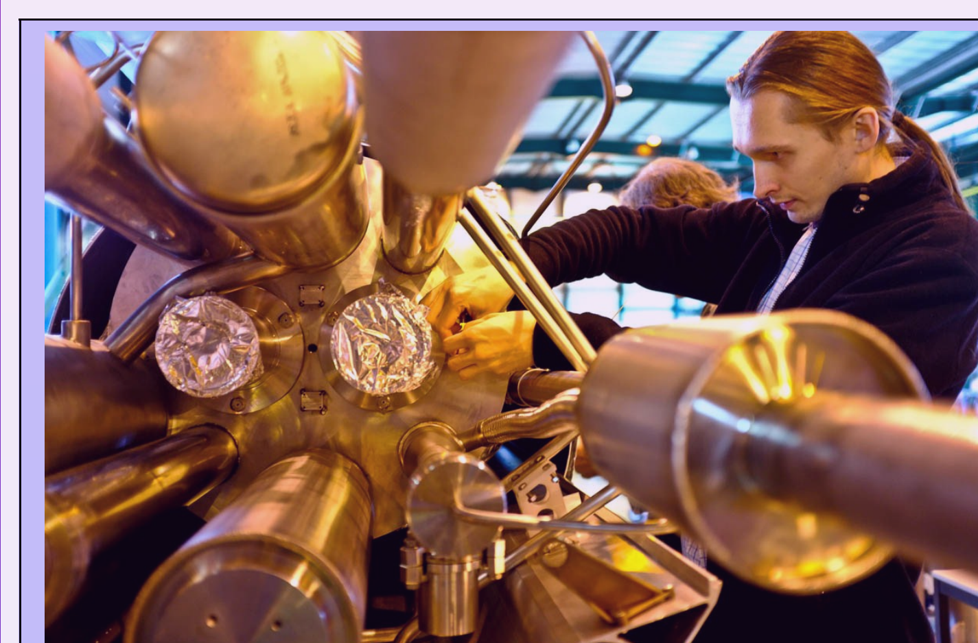
Figure 16: Installation of cryogenic particle detector on the cold mass of LHC magnet.
