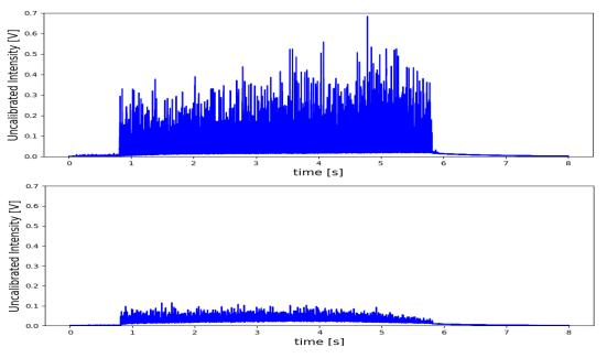
Extracted beam intensity over time, 50kHz sampling. (top) Reference (bottom) with RF-channeling. Same integrated intensity, or comparable with shot-to-shot variations.
