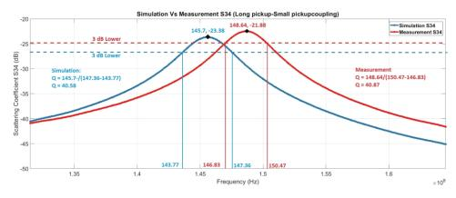
Comparison of Scattering parameter S34 between a long and a short pickup between simulation and measurement
