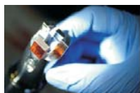
Photograph of an electro-optic GaP crystal, mounted on its support. Image courtesy of Nicole Hiller, KIT, Germany
