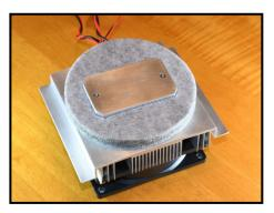
**Figure 6** Aluminium cold plate
