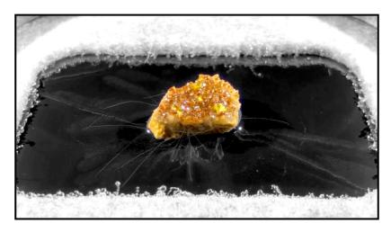
The image above shows a sample of the mineral boltwoodite that contains some uranium. The narrow tracks are beta particles (electrons) and the broader, more ghostly, tracks are alpha particles (nuclei of helium atoms). The image is a composite made from about 30 still frames extracted from a one-minute video.
