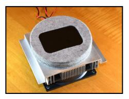
**Figure 7** Black plate on cold plate
