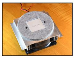
**Figure 4**Peltier module surrounded by a felt coaster
