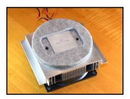
**Figure 5**Second Peltier module stacked onto first
