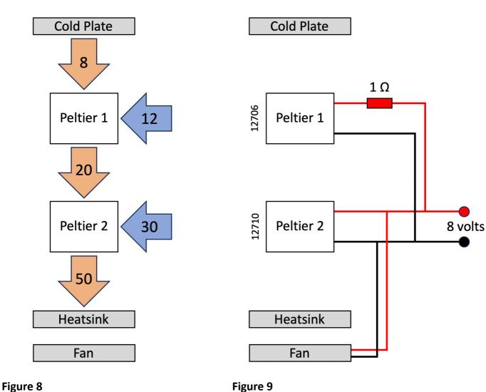
Heat flow (orange) between the cold plate and the heatsink and electrical power (blue) supplied to the Peltier
