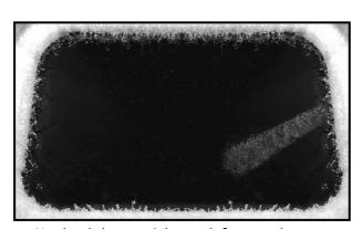
Single alpha particle track from radon gas
