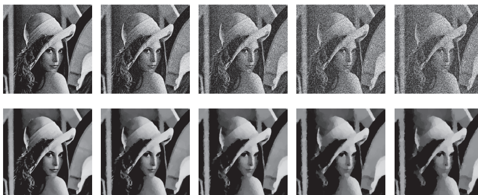
FIG. 4.6. Numerical results of Lena test image with different variance \sigma^2 . From left to right on the first row: noise image of variance, respectively, \sigma_1^2 = (\frac{20}{255})^2 \times 512^2 (or psnr = 21.87 ), \sigma_2^2 = (\frac{40}{255})^2 \times 512^2 (or psnr = 15.85 ), \sigma_3^2 = (\frac{60}{255})^2 \times 512^2 (or psnr = 12.33 ), \sigma_4^2 = (\frac{80}{255})^2 \times 512^2 (or psnr = 9.83 ), and \sigma_5^2 = (\frac{100}{255})^2 \times 512^2 (or psnr = 7.89 ). From left to right on the second row: the associated restoration results and corresponding psnr s : 29.35, 26.50, 24.98, 23.95, 23.16.
