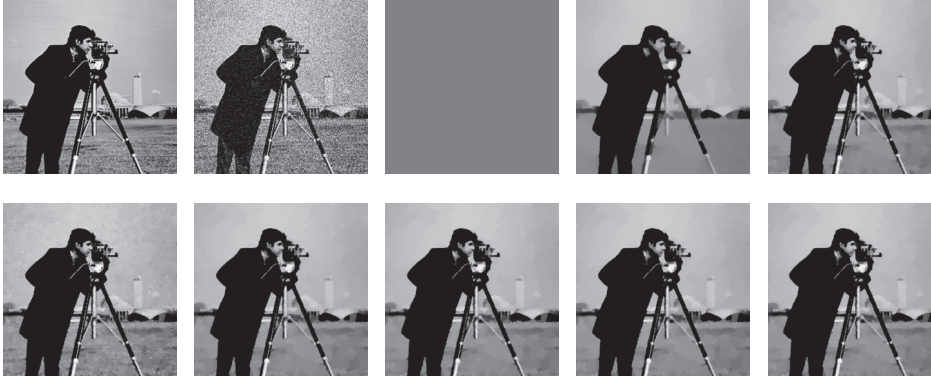
FIG. 4.5. Camera image denoising result. From left to right and then top to bottom: the original image, the noisy image with a zero mean Gaussian random noise of variance \sigma^2 = (\frac{50}{255})^2 \times 512^2 (or \text{psnr} = 14.30 ), and eight restoration images: mean image by setting \lambda = 0 , the denoised image from setting \lambda = M = 1000 , and the denoised image sequence at multiplier \lambda_k ( k = 1, \dots, 6 ); the \text{psnr} of the final image is 27.17.
