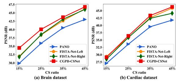
Fig. 4. Performance comparisons on Cartesian under-sampled k-space datasets with untrained CS ratios for brain dataset (a) and cardiac dataset (b). "-Left" denotes the reconstruction of untrained CS ratio 15%, 25%, 35%, 45% sampled data with trained models of CS ratios 10%, 20%, 30%, 40%, respectively. "-Right" denotes the reconstruction of untrained CS ratio 15%, 25%, 35%, 45% sampled data with trained models of CS ratios 20%, 30%, 40%, 50%, respectively.
