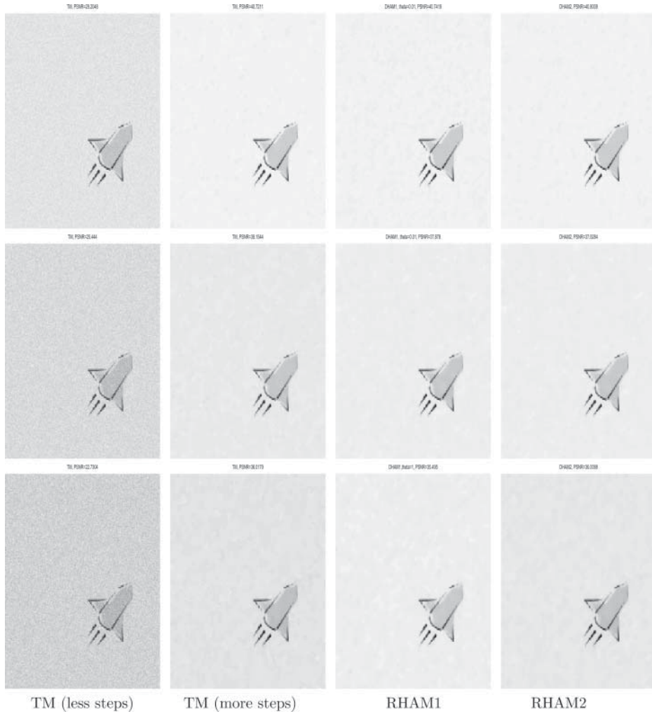
Figure 4. Test Set-1 Example 4. From the top row to the bottom, 10%, 15% and 20% random noise has been added to the image. For each row, the first image shows the result obtained with the TM method for the same number of iterations as the maximum iterations used for RHAM1 and RHAM2, the second image shows the result obtained with the TM method, and the third and fourth images show the results obtained for RHAM1 and RHAM2.
