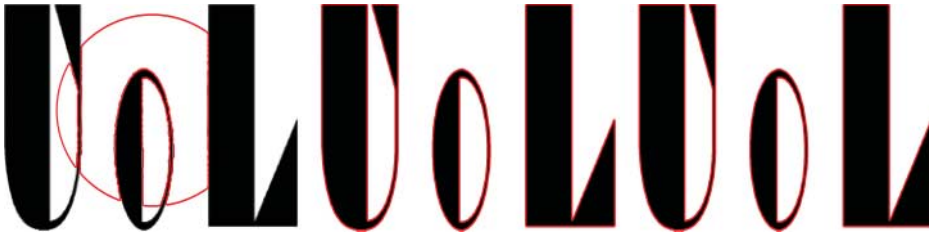
Figure 8. Test Set-1 Example 3. Successfully reached relative residual equal to 10^{-2} after 9 iterations for RHAMs and 186 iterations for TM. (a) TM method result after 9 iterations, (b) HAM1 method result after 9 iterations and (c) HAM2 method result after 9 iterations (colour online only).
