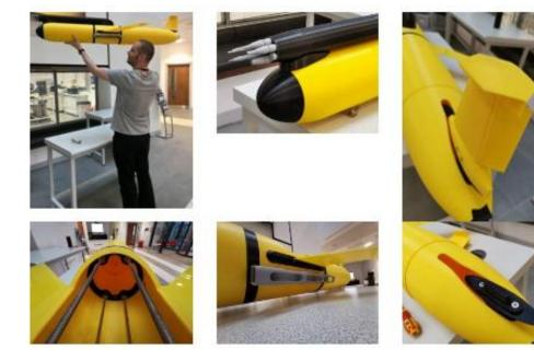
Project demonstrates rapid prototyping facilities and illustrates the capabilities at Sensor City to make things far larger than the normal scope of a 3D printer
