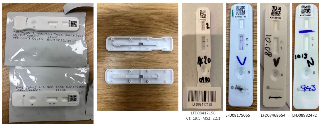
Figure 8: Examples of device build differences and reading issues
