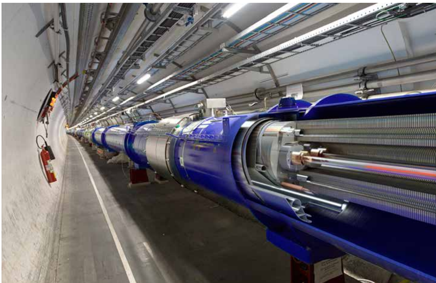
Cross-section of one of the Large Hadron Collider dipole magnets
