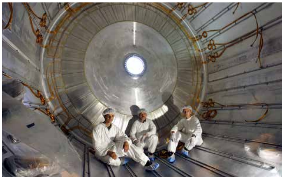
Three scientists with one of the end-caps of the ATLAS detector, which will be used to detect particles produced in proton-proton collisions
