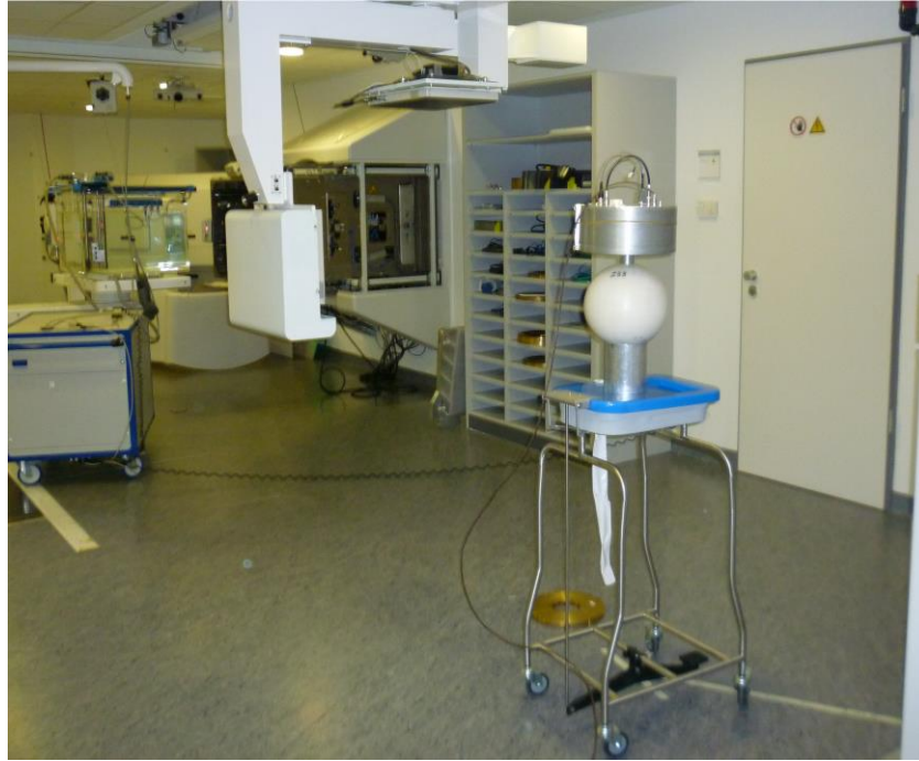
FIG. 45. Experimental set-up for the measurement performed with the 233 mm sphere in position 1a at the Essen proton therapy centre.
