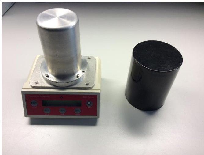
FIG. A10. Picture of ABC bubble detector (left) and the additional lead shell (right).
