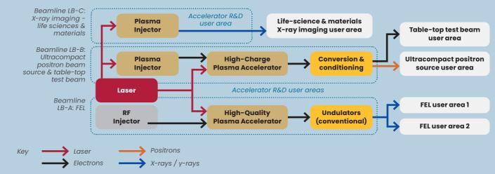
These layouts require a floor space at least a factor 3 smaller than that needed by conventional RF accelerators. EuPRAXIA plans to reduce the facility size even further throughout its lifetime. Up to a factor of 10 reduction in size could be achieved through additional improvements and implementation of novel beam transport technologies, diagnostics and other key components.
