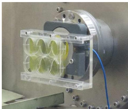
Experimental setup for the irradiation of radiochromic films. The picture shows the kapton window, the ionization chamber and the holder for the film mounted together at the end of the beam line.
