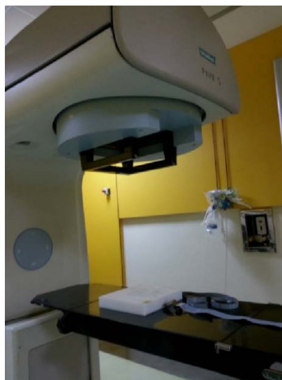
The detector installed inside a slab phantom, at the Virgen Macarena Hospital, positioned for irradiation by a clinical linac.
