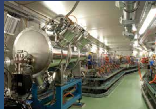
Superconducting Wiggler at ALBA.
