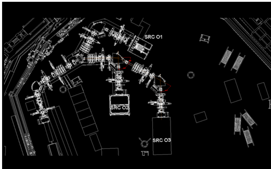
Possible layout of the INSPIRIT ion source inside the CNAO synchrotron, Courtesy of S. Sironi
