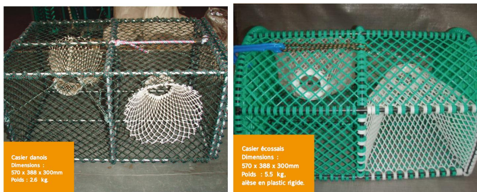
Fig. 5.2.6.1.1 Danish and Scottish creels used in the PRESPO project study on the feasibility of Nephrops creels in the Bay of Biscay (Source: Figarede et al., 2011).
