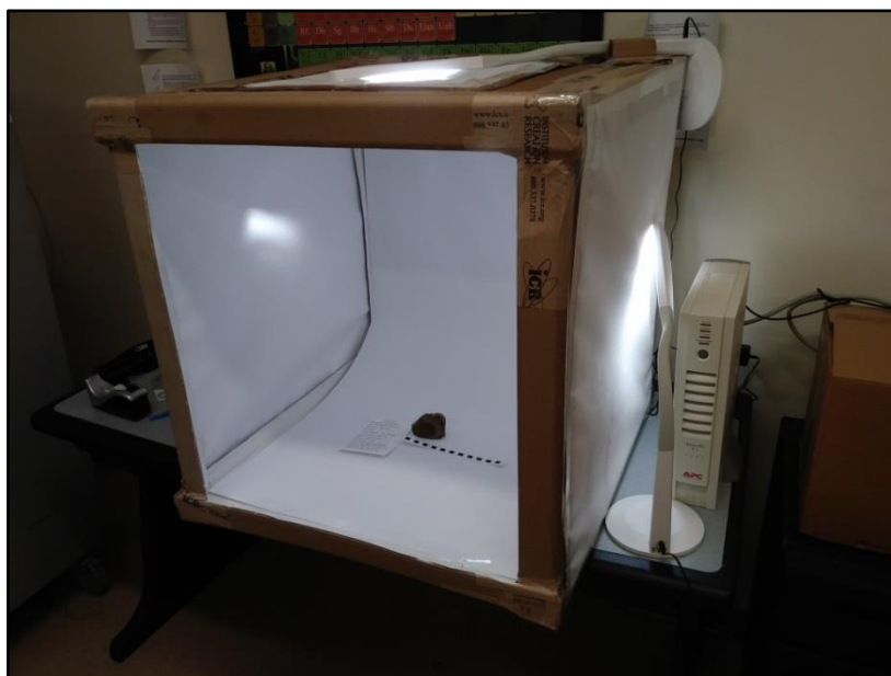
Figure 2.14 | Light box. Construction of a light box was essential to achieve optimum lighting for sample photography of each suitable fossil fragment on loan.
