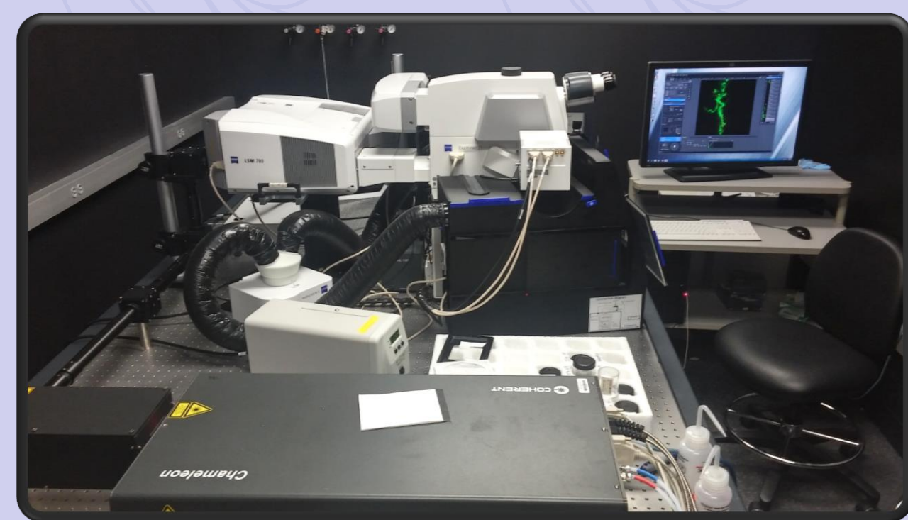
Fig. 2. Zeiss Examiner Z1 two-photon excitation laser scanning confocal microscope coupled to a Coherent Chameleon titanium: sapphire laser at UT Southwestern Medical Center Live Cell Imaging facility.
