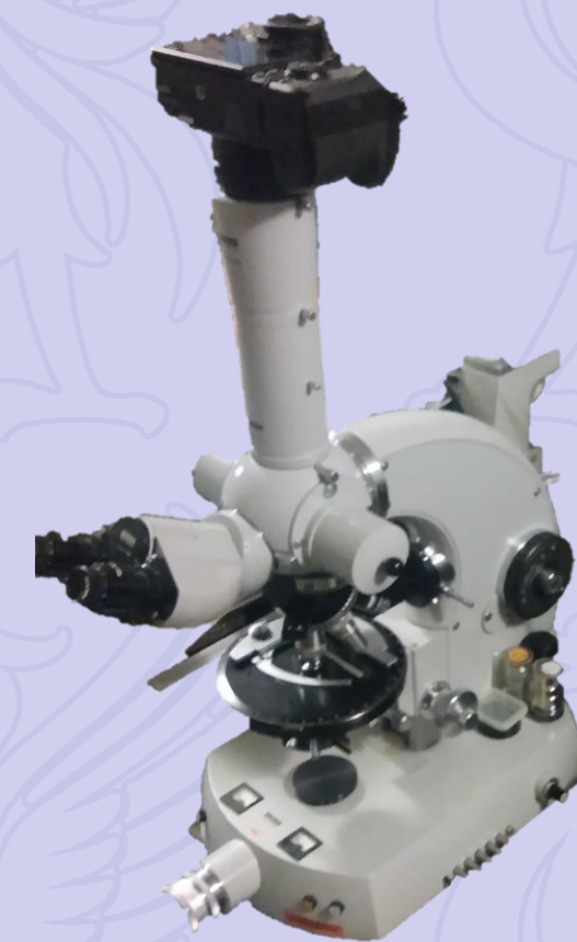
Fig. 1. Zeiss Photomicroscope with 1 st order red filter and Panasonic Lumix S1 digital full frame camera
