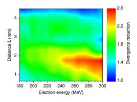
The colour map shows the factor of reduction of the divergence, as a function of the electron energy and of the distance *L* between the accelerator and the lens. The peak electron density in the focusing stage is  $^{3.9} \times 10^{18}$  cm<sup>-3</sup>.
