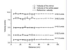
Example of measurements from the experiments using a movable stage, which allows for a precise velocity measurement (straight solid line) in the range of 0.01 to 10.00 cm/s with a mirror (dot lines) and white paper (thick solid lines) with an error bar obtained at different distances between the laser and the target.
