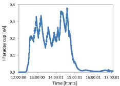
Ion current accumulated for  $^{124}$ Sn during the efficiency measurement (The total integrated ion current compared with the known amount of atoms in the original sample) with a result of  $4.53\pm0.09\%$ .
