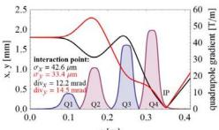
Final focus system with continuous gradients from 3D models, emittance=  $13\pi$  mm mrad,  $\delta E$ =0.01.
