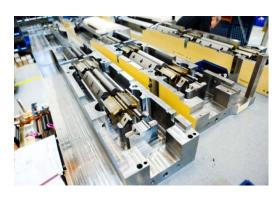
Compact magnet systems are smaller and thus the number of elements can be increased. This results in an extremely low emittance. The low emittance makes possible an extremely bright synchrotron light.
