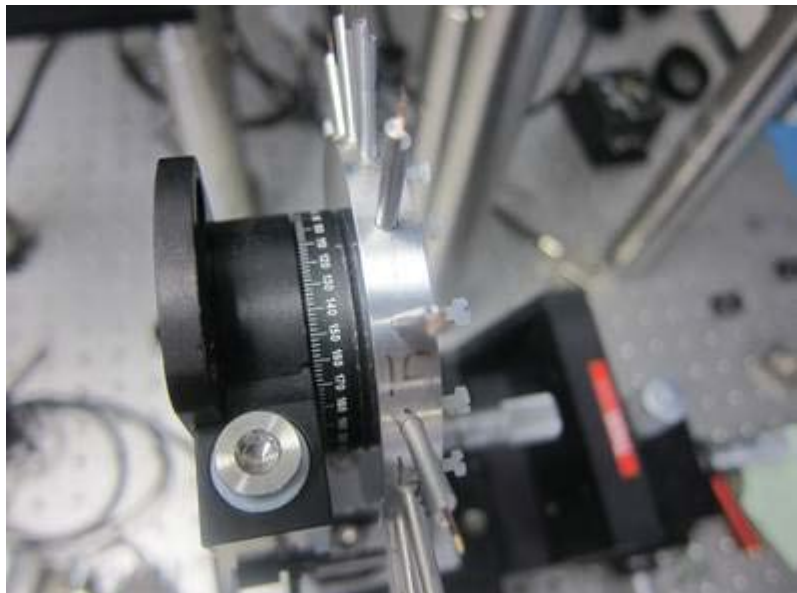
Target wheel holding the ultra-thin targets employed in the experiment.
