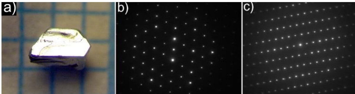
Figure 1: icosahedral approximant Al 65 Cu 18 Co 7 Fe 10 : single crystal (a) and SAED parents along the threefold (b) and twofold (c) zone axes.
