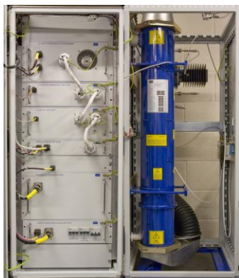
S-Band 50 kW transmitter PTX7610, incorporating high reliability travelling wave tube
