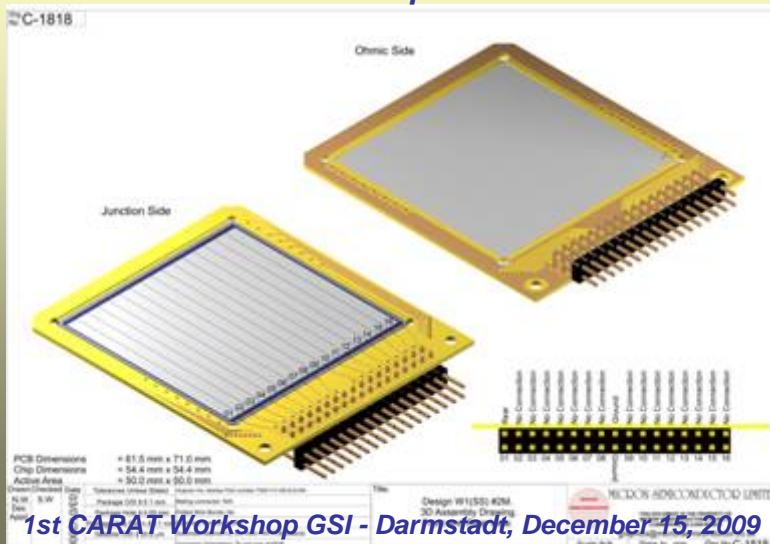
Micron Semiconductor Area 50 mm x 50 mm Thickness 500 microns 16 strips
