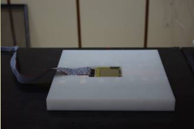
Micron Semiconductor Area 50 mm x 50 mm Thickness 500 microns 16 strips
